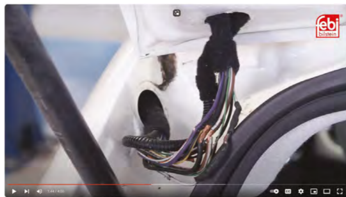
[EN] Fiat 500 tailgate wiring harness repair febi bilstein 17.6K subscribers 71 views
